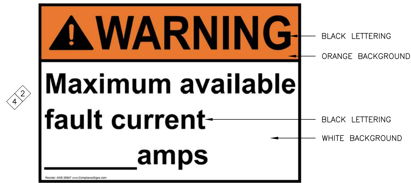
COMPLIANCE SIGNS #AWE-26847, 5" X 3.5" CONTRACTOR SHALL FILL IN AVAILABLE FAULT CURRENT (AFC) VALUE FOR EACH PANELBOARD, SWITCHBOARD AND SWITCHGEAR, USING VALUES SHOWN ON SINGLE LINE DIAGRAM(S)
