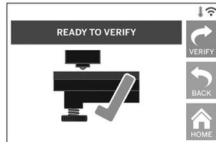
7. Repeat steps 4-6 for the second position, when bed is fully level the extruder will automatically move to the calibration position and complete the leveling process.
