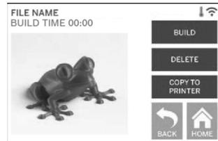
5. Your 3D40 will first align the extruder and build platform to their zero positions then the level sensor will lightly touch the build plate to complete alignment. Your extruder tip will begin to heat which may take a few minutes. Once the proper temperature is reached your model will begin to build.
